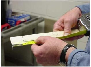
One method to insure accurate mix ratios is to put measurements on sticks with the appropriate mix ratio. In the case of the 315BC and 315TOP this is 2 Parts A to 1 Part B, so you might do 2 inches "A" to 1 inch of "B"
